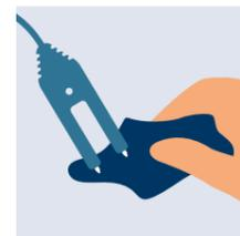
Check the water sensor's measuring tips at regular intervals. If necessary, clean the metal ends with a damp cloth. Check regularly to see if the WD 1000 device is working properly by bridging the water sensor with a metal part.
